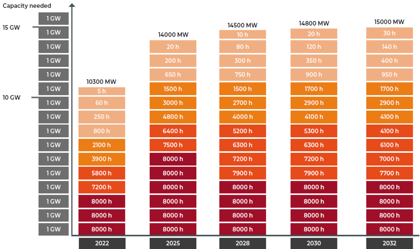
Figuur 13 Residual load for Belgium; during how many hours is a certain capacity required, in addition to RES and nuclear capacity according to 'central' scenario, Eliä, fig. 5-3, p.166
